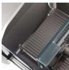
Remnant holder and hand guard on same level
